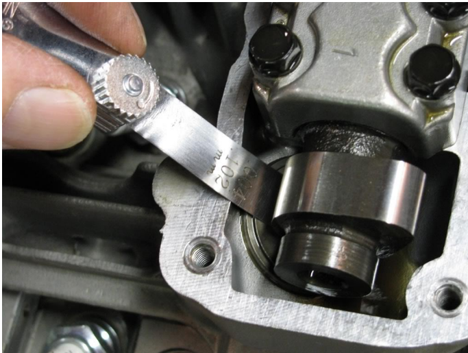
How to measure tappet clearance.
