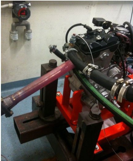
Figure 10 - The KTM SX-F stock engine in the dynamometer room at Monash University.
