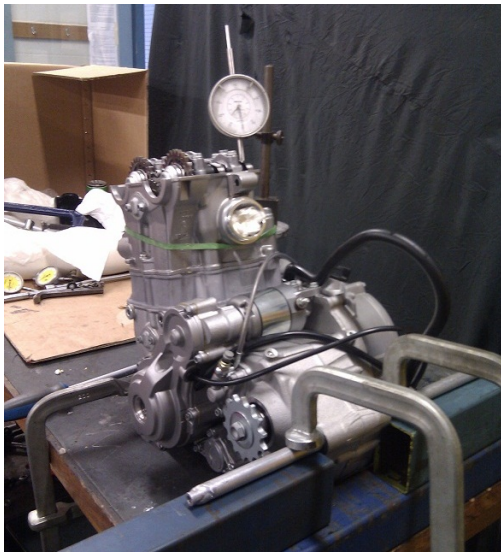
Figure 18 - The valve profiles were manually measured at Monash University.
